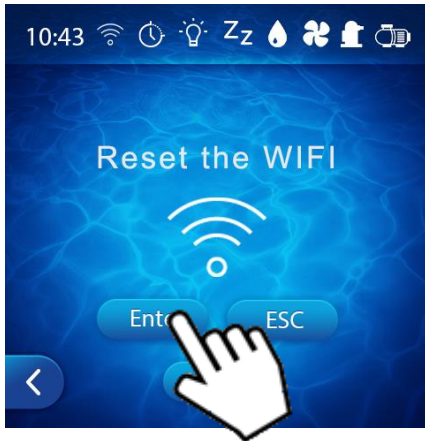
Press the button Enter on the Wifi screen of the display
