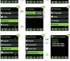
**6.9** Sound: Programming of the system to emit sound for the functions: **Keyboard** (keys); **Notices** (pop-up message); **Alarms** (working alarm); **Filtration** (start of the filtration).
